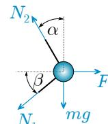
$$\begin{aligned}\sum Y &= 0 \rightarrow N_2 \cos \alpha - N_1 \sin \beta - mg = 0 \rightarrow \\ &\rightarrow N_2 = \frac{mg}{\cos \alpha} = \frac{100}{\cos 30^\circ} = 115.5 \text{ N}, \\ \sum X &= 0 \rightarrow F - N_2 \sin \alpha = 0 \rightarrow F = N_2 \sin \alpha = 57.7 \text{ N}.\end{aligned}$$
