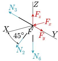
$$\begin{aligned}\sum X = 0 \quad &\rightarrow \quad F_X + N_2 \frac{\sqrt{2}}{2} = 0 \quad \rightarrow \quad F_X = -\frac{\sqrt{2}}{2} = -0.707 \text{ kN}, \\ \sum Y = 0 \quad &\rightarrow \quad F_Y - N_3 = 0 \quad \rightarrow \quad F_Y = 1.000 \text{ kN}, \\ \sum Z = 0 \quad &\rightarrow \quad F_Z - N_6 - N_2 \frac{\sqrt{2}}{2} = 0 \quad \rightarrow \\ &\rightarrow \quad F_Z = \left(1 + \frac{\sqrt{2}}{2}\right) = 1.707 \text{ kN}.\end{aligned}$$
