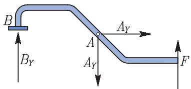
$$\begin{aligned} \sum X &= 0 \quad \rightarrow \quad A_X = 0, \\ \sum M_Z^B &= 0 \quad \rightarrow \quad F 2a - A_Y a = 0 \\ &\rightarrow \quad A_Y = 2F = 0.4 \text{ kN}. \end{aligned}$$
