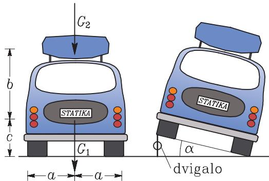
$$G_1 = 6 \text{ kN}, G_2 = 1 \text{ kN}, a = 0.8 \text{ m}, b = 1.2 \text{ m}, c = 0.5 \text{ m}.$$
