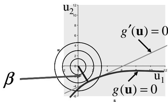
Figure 2      Illustration of the linearization proposed by Hasofer and Lind [3] in standard normal space.
