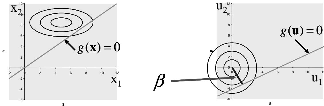
Figure 1 Illustration of the two-dimensional case of a linear limit state function and standardised normally distributed variables  $\mathbf{U}$ .
