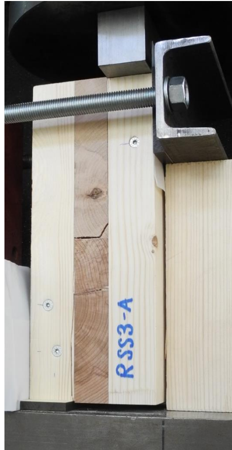
Compression shear tests with hybrid beech CLT stripes
