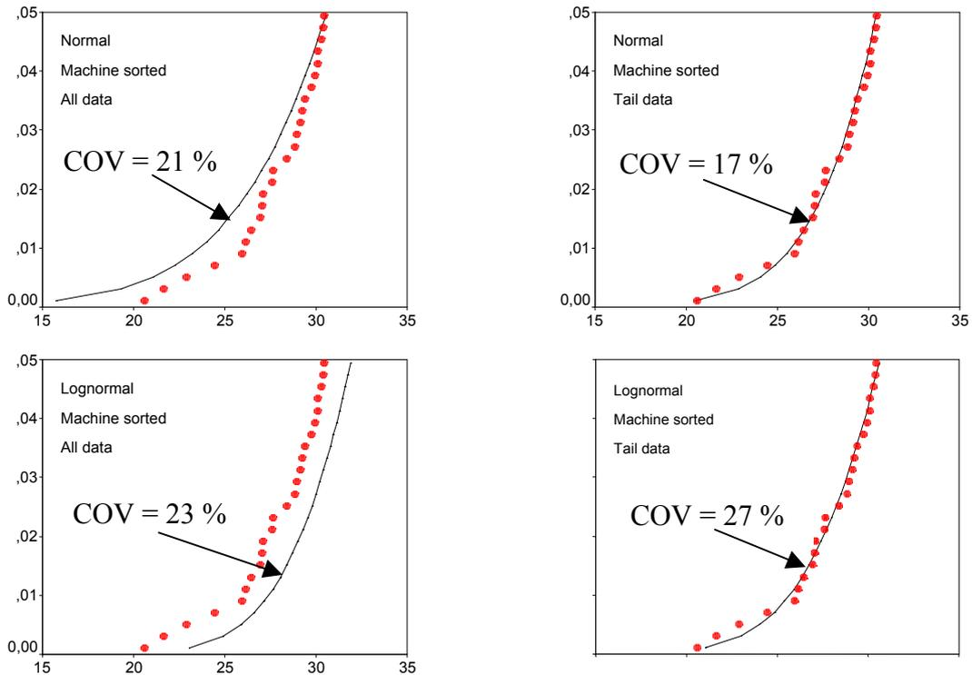
Figure 3. Cumulative distributions of bending strength for machine sorted spruce of dimensions 42 x 146 mm. The spruce was sorted by Raute Timgrader to the European strength class C30. The coefficient of variation values are given for the distributions, showing high values for the tail-fitted log-normal distribution.
