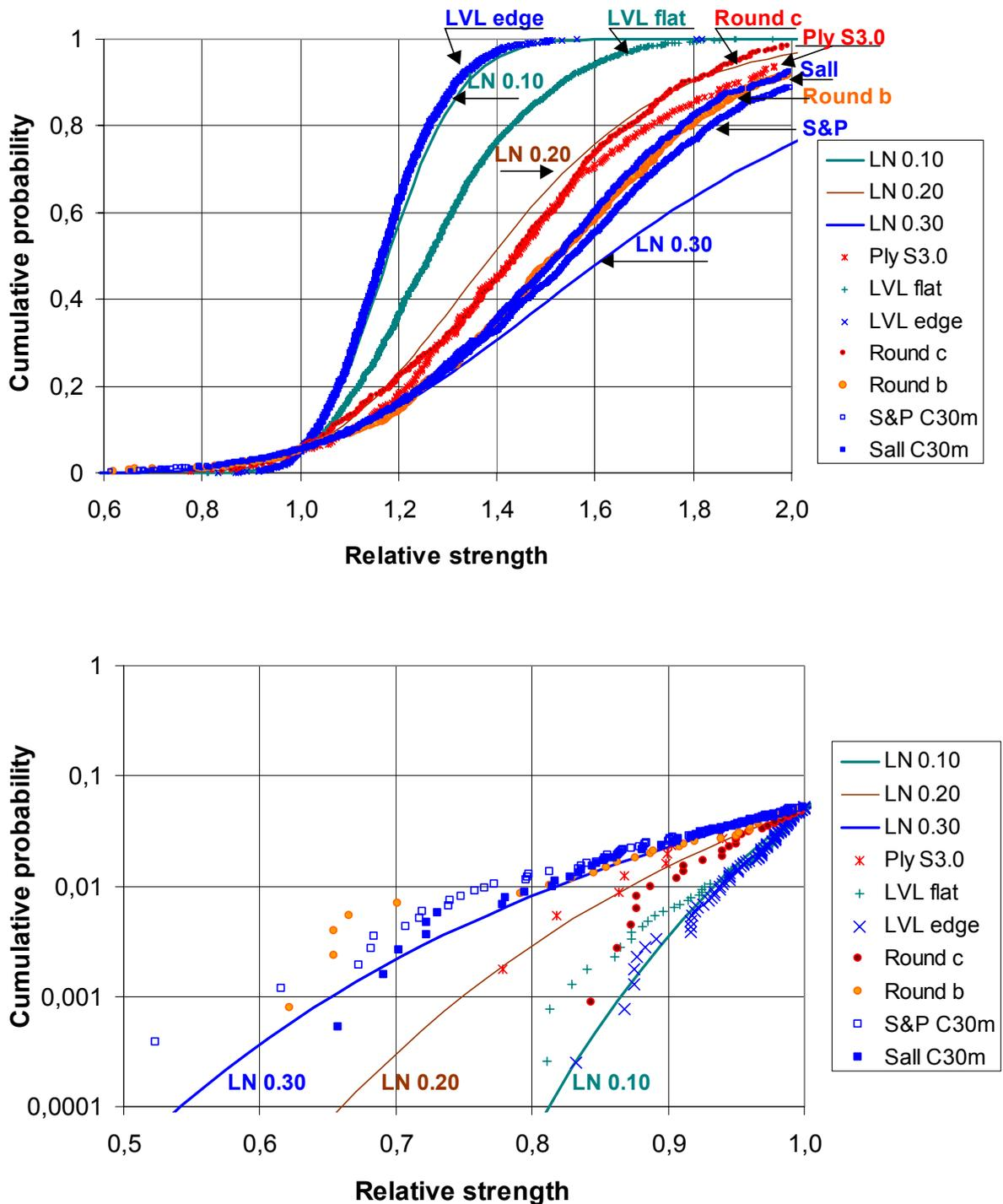
Figure 2. Cumulative probability distributions of relative strength (strength per 5<sup>th</sup> percentile) of sawn and round timber, LVL and plywood on linear and logarithmic scale as well as log-normal function with  $COV = 0.1, 0.2, \text{ and } 0.3$ .
