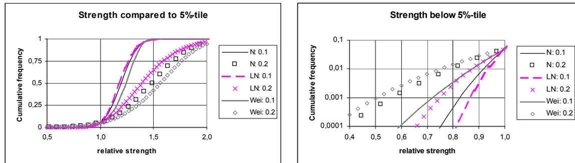
Figure 1. Comparison of Normal (N), Log-normal (LN) and 2-parametric Weibull (Wei) distributions when coefficient of variation is 10 or 20%, the number following N, LN or Wei is the coefficient of variation, Ranta-Maunus et al.(2000)
