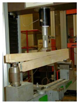
In order to validate the empirical formulation, finite element simulations are realised. The main interest is to model with simple considerations about ultimate characteristics of wood and adhesive, the simultaneous crack propagation in timber and the damage of the glued interface.
