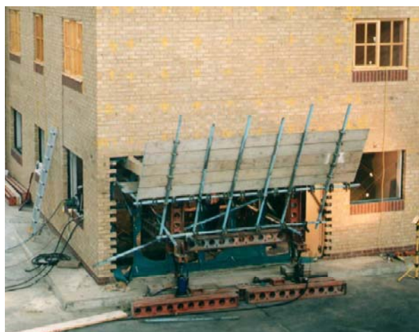
Figure 5: Disproportionate Collapse Test
