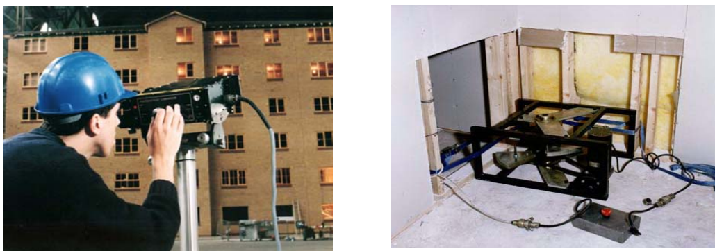
Figure 8: Stiffness measurements of the TF2000 building
