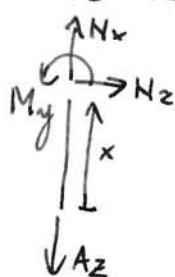
$$\begin{aligned} N_x = A_z = -7 \text{ kN} \\ N_z = 0 \\ M_y = 0 \end{aligned}$$
