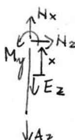
$$\begin{aligned} N_x = A_z + E_z = -3 \text{ kN} \\ N_z = 0 \\ M_y = 0 \end{aligned}$$
