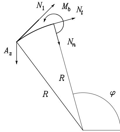
$N_t = 1/4 F (3 \sin(\varphi) - \cos(\varphi))$ ,  $N_n = 1/4 F (3 \cos(\varphi) + \sin(\varphi))$ ,  $M_b = -5/4 F a (-3 - \cos(\varphi) + 3 \sin(\varphi))$ ,
