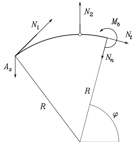
$N_t = 1/4 F (3 \sin(\varphi) + \cos(\varphi))$ ,  $N_n = -1/4 F (-3 \cos(\varphi) + \sin(\varphi))$ ,  $M_b = -5/4 F a (-3 + \cos(\varphi) + 3 \sin(\varphi))$ .
