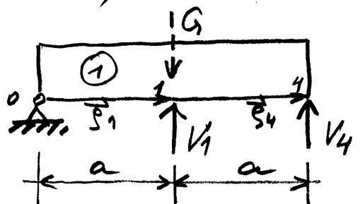
$$\vec{u}_0 = \vec{0}, \quad \vec{\omega}_0 = \omega_y \vec{e}_y \\ \vec{p}_1 = a \vec{e}_x, \quad \vec{p}_4 = 2a \vec{e}_x$$
