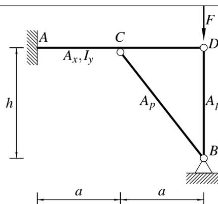
**Podatki:**  $F = 5$  kN,  $a = 3$  m,  $h = 3$  m,  $A_p = 200$  cm<sup>2</sup>,  $A_x = 200$  cm<sup>2</sup>,  $I_y = 5000$  cm<sup>4</sup>,  $E = 200\,000$  MPa.
