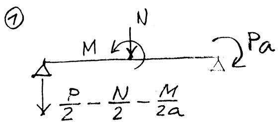
$$M_y = -\left(\frac{P}{2} - \frac{N}{2} - \frac{M}{2a}\right)x - N(x-a) - M(x-a)^{\circ} = -E I_y w$$
