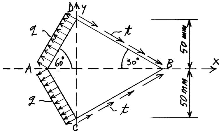
$$\begin{aligned}a &= 50 \text{ mm} \\q &= 120 \text{ MPa} \\E &= 200\,000 \text{ MPa} \\v &= 0.3\end{aligned}$$
